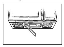
Be sure bulbs to be replaced are cool before removing. Break the adhesive seal by gently unscrewing the bulbs. Replace with 40-watt incandescent bulbs (Part No. WB02X4253) available from vour GE supplier. 'High intensity 40-watt bulbs (Part No. 40S11N/1) which are available in supermarkets and hardware stores may also be used for replacements. Raise light compartment cover and replace screw. Connect electrical power to microwave oven.
